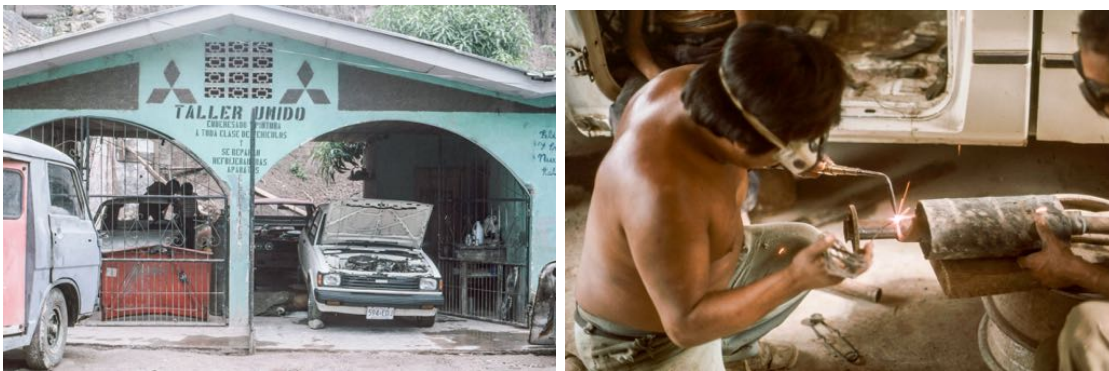
Figure 683. Fixing our exhaust pipe.
