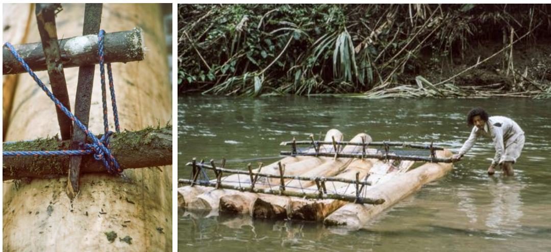
Figure 1005. Ironwood wedges enter the balsa trunks easily for holding the raft together.
