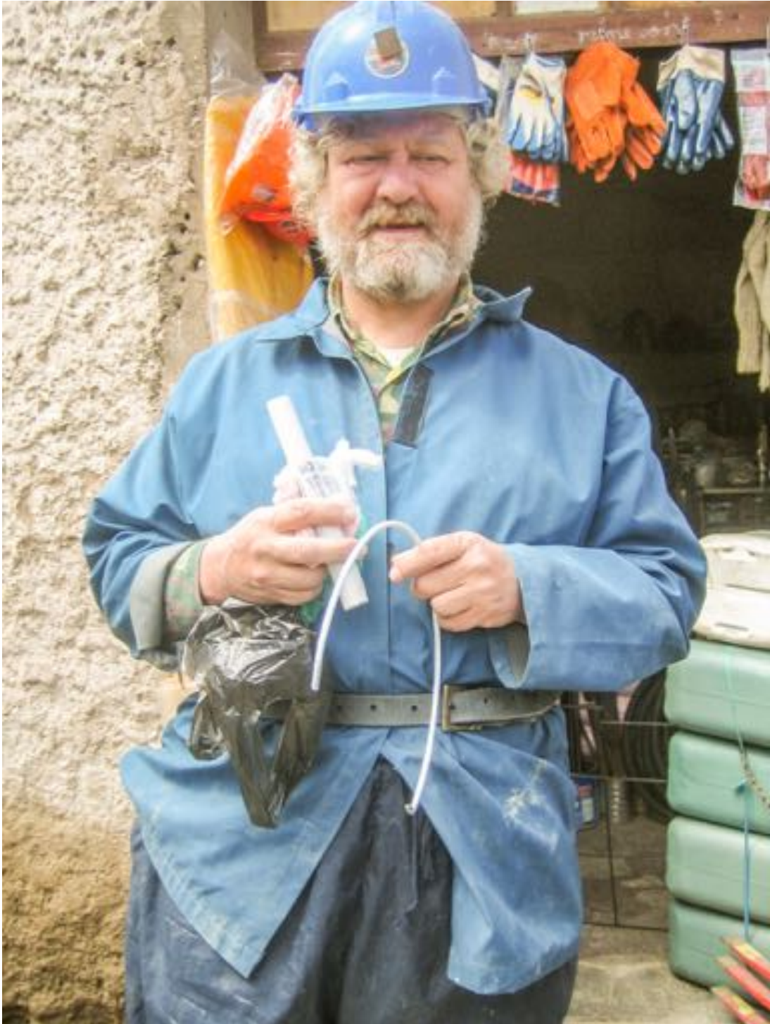
Figure 1160. Fully equipped with dynamite stick, fuse, ignition cap, helmet.
