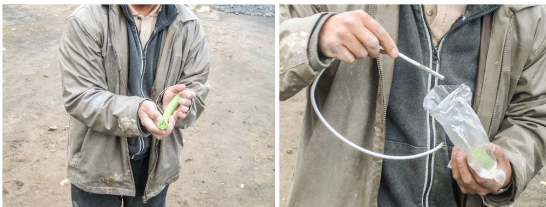
Figure 1164. The guide molding my dynamite and inserting the fuse.
